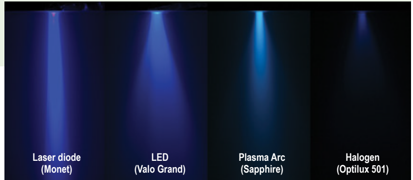
Beam comparison of four curing lights: The Monet laser exhibited an intense collimated beam while other light sources had greater beam divergence and diminishing energy.
